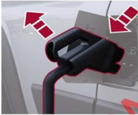
Removing The Charger Connector From The Vehicle Charge Inlet
